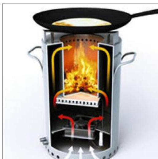
Figure 3: Forced draft rocket ICS with top fuel intake
