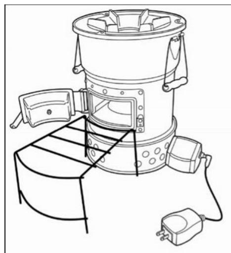
Figure 4: Forced draft rocket ICS with lateral fuel intake
